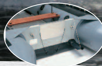
Heavy-duty bailer and aluminum-plated transom
