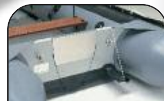
Heavy-duty bailer and aluminum-plated transom
